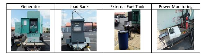
For each generator tested, a known amount of untreated fuel was run through the generator, and the liters of fuel consumed per hour and kW-Hours of electricity generated determined. Then the same was done with fuel treated with ENVIRO-KLEENZE<sup>™</sup>. The difference in L/kW was calculated as Improvement %.
